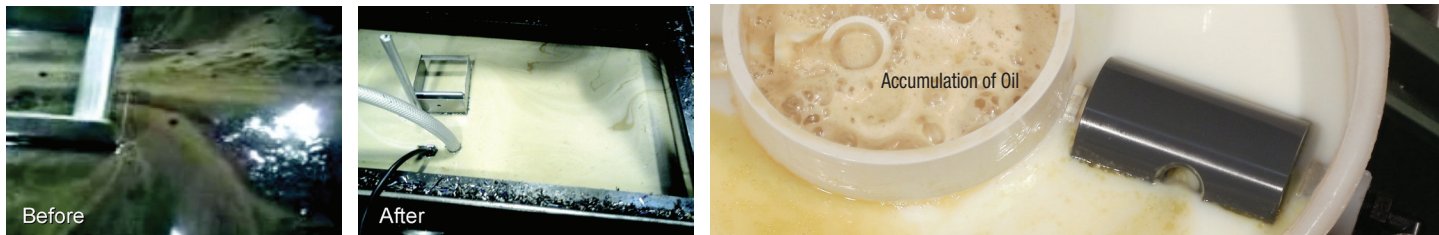
Flexor in action, with Sumpster, removing tramp oil (and a glob of biofilm), cleaning A neglected sump in under two hours.
