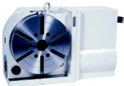
Model 220 with digital AC servo motor
