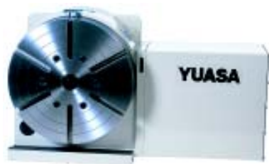
Model DRFT-320 with Fanuc AC servo motor
