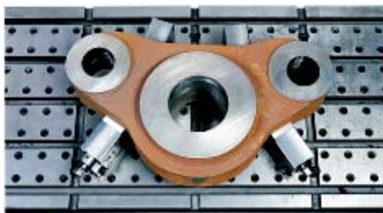
The photo above shows two stationary blocks and two movable blocks arranged around the part.
