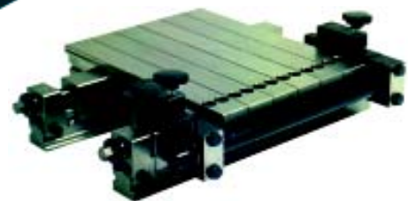
Multiple parts aligned with bar-type work stop.
