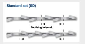
All-purpose set for cutting thicknesses of more than 0.2 inch with steels, castings and hard non-ferrous metals.
