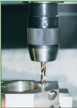
1 Drill coolant passage, leaving reaming allowance.
