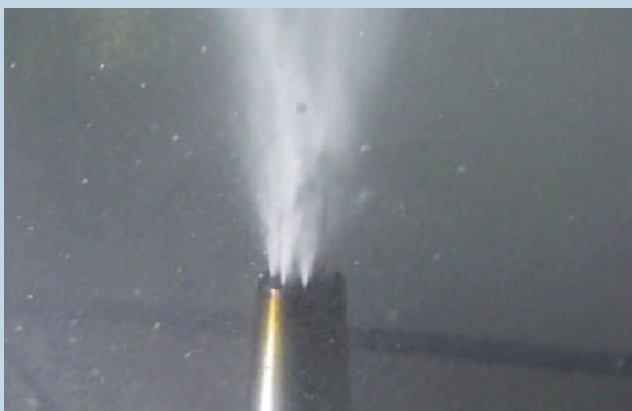
Cool Flash – effective cooling at the cutting edges
