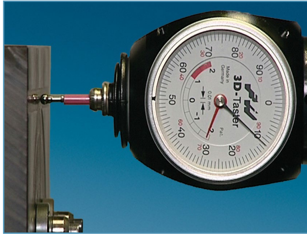
Tram in your work piece or fixture to your machine
