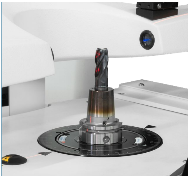
Non-contact measurement with a high-resolution camera and digital image processing, incl. measuring software "Microvision"
