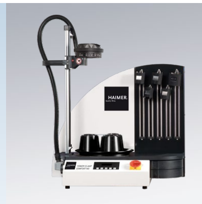
Power Clamp Profi Plus NG High powered shrink fit machine – Heating power 20 kW – For shrinking of tools from \varnothing 1/8" - 2" (3 – 50 mm) – For HSS- and solid carbide tools – Big coil for \varnothing 1\frac{1}{2}" - 2" (40 – 50 mm) optional – Incl. rotary table and chuck support – Incl. tool tray – With craning boxes for accessories
