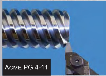
ACME EXTERNAL THREADING 4 THREADS PER INCH AND GREATER
