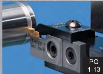
1.000" DEPTH OF CUT 2, 3, 4, 5 AND 6MM INSERT WIDTHS
