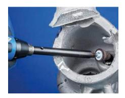
Mounted points with a shank diameter of 1/8" and 1/4" can be extended with drive spindle extensions. They allow access to hard-to-reach areas. The drive spindle extension is mounted in the collet of the power tool (air grinder or electric grinder), or in the handpiece of the flexible shaft. In some applications, spindle extensions are an economical alternative to customized mounted points with long shanks.
