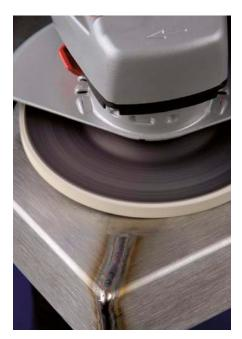
Poliflex® wheels with the textile (TX) bond are manufactured with standard aluminium oxide. The textile fabric inlays make the TX bond a very hard, sturdy bond. Recommended for use on edges.
