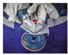
Release the disc by using the lever.
