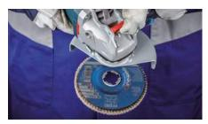
Release the disc by using the lever.
