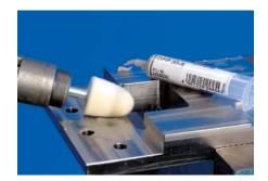
Diamond polishing pastes are used for work on hard materials, such as tungsten carbide and hardened steels. They are used in combination with felt polishing elements. Diamond polishing pastes can be diluted and dissolved with water and alcohol.
