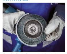
Place the disc on the X-LOCK holder in a formfitting manner.
