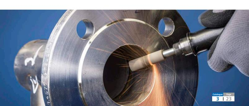
For edge grinding on stainless steel (INOX)
