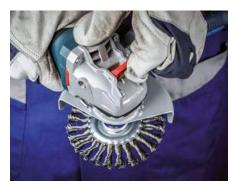
Release the brush by using the lever.
