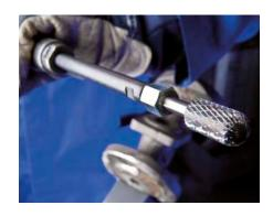
Burs (shank dia. 1/8, 1/4 and 3/8 inch) can be extended with spindle extensions. They allow access to hard-to-reach areas. The drive spindle extension is mounted in the collet of the power tool (airpowered or electric), or in the handpiece of the flexible shaft drive. In some applications, spindle extensions are an economical alternative to customized extended shank burs.
