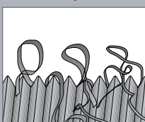
Poor Chip Control
