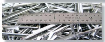
The HV11's long length creates lengthy, needle-like chips in aluminum.
