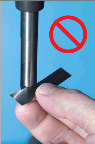
Figure 3a. Shim should NOT enter intersection
