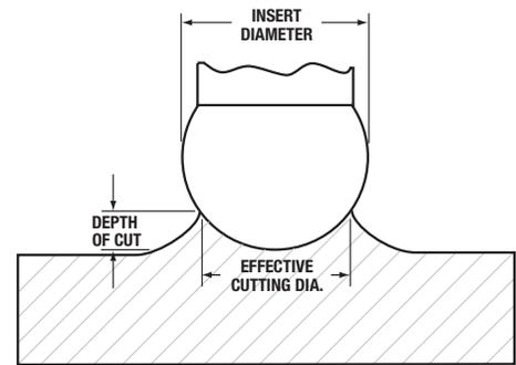
\* For the cuts that are not strictly tip-cutting, but will use both the tips and sides of the SBN insert, pick an effective cutting diameter in between the ECD in the chart and the actual diameter of the insert. For example: If the ECD comes out to .210" with a .750" diameter insert, use .480" as your ECD when calculating RPM.
