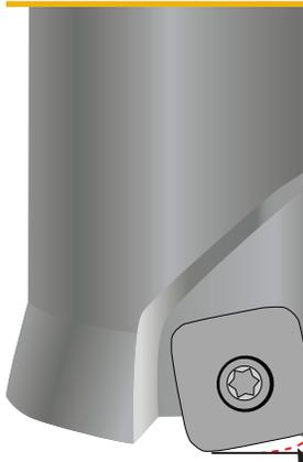
Mid-feed inserts have a stronger cross-section than the mini-feed, but are smaller than the heavy-feed. These are great general-purpose inserts best suited for lighter-duty (40-taper, linear ways, etc.) machines. Run faster feeds with lighter DOC in most situations. In heavier DOC, run the lower to middle area of the feed ranges.
