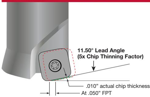
High-feed milling creates significant chip thinning due to an extreme lead angle. Feed rates must compensate for this to maximize productivity. The figure at left shows an example of this condition. Adjusting feed rates to account for chip thinning creates cutting conditions that provide very high feeds (IPM), but at lighter depths of cut (DOC). See the specific instructions for each size of high-feed insert to get the most out of your Dapra RHINO-FEED product!
