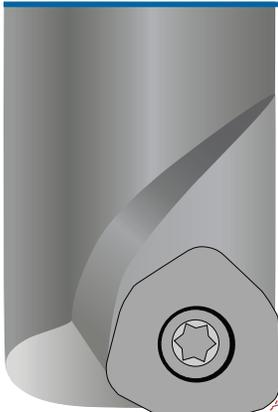
Mini-feed inserts have the smallest IC (Inscribed Circle) and smallest cross section. It is suggested to run a good common-sense combination of feed and DOC with these inserts. When running a light DOC, the higher end of the feed range is acceptable. When running heavier DOC, use the lower to middle feed ranges. Index inserts promptly upon visible wear to avoid breakage.
