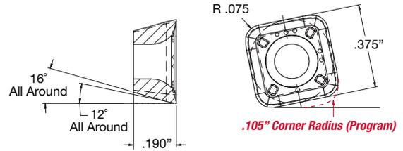
\*A special corner radius value is required for correct programming of a high-feed insert. Using the program radius avoids gouging of the corners in the workpiece material. The high-feed insert will naturally leave a small amount of extra material at the bottom-most layer of the cut, at the intersection of the wall and pocket floor. See diagram at bottom of this page.
