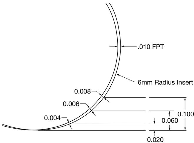
This diagram (left) shows the varying chip thickness when feeding .010" feed per tooth (FPT) at different depths of cut (DOC) with a 12mm diameter insert:
