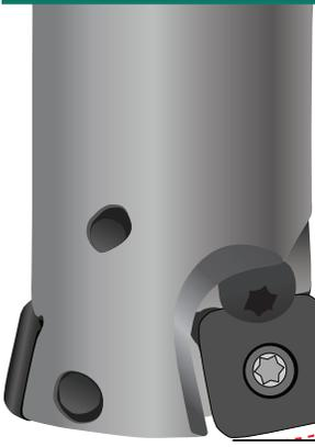
Heavy-feed inserts have the strongest cross-section of the RHINO-FEED line. Heavy-feed inserts are suitable for heavier DOC and larger machines (50-taper, box ways, etc). For optimum performance, use good combinations of heavier DOC with light-to-middle FPT, or lighter DOC with heavier FPT.
