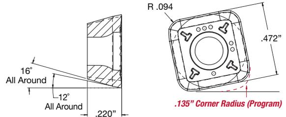
\* A special corner radius value is required for correct programming of a high-feed insert. Using the program radius avoids gouging of the corners in the workpiece material. The high-feed insert will naturally leave a small amount of extra material at the bottom-most layer of the cut, at the intersection of the wall and pocket floor. See diagram at bottom of this page.
