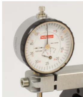
Dial gauge with an accuracy of 1/100 mm.
