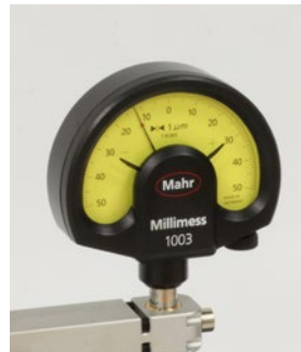
Dial gauge accurate to the \mu\text{m} (1/1000 mm) with reduced measuring force.
