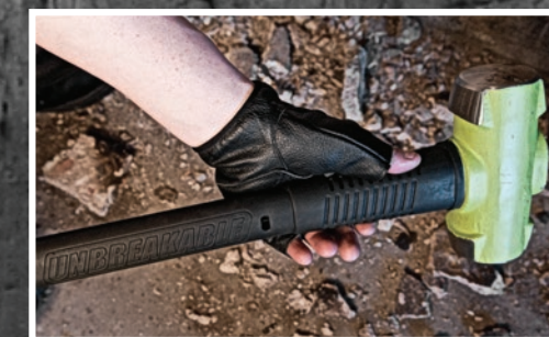
ANTI-VIBE NECK ERGONOMICALLY DESIGNED TO PREVENT INJURY FROM REPEATED JOB SITE USE
