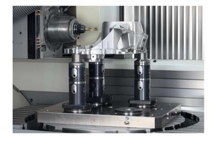
4 double clamp basic modules positioned on a tooling plate. Optimum 5-side machining is possible.
