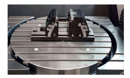
Mounted directly on a KIPP zero-point clamping system over the integrated clamping bolts in the vice base plate.
