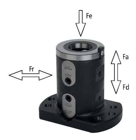
Fr Permissible transverse force Fa Permissible clamping force Fd Permissible contact force Fe Clamping bolt pull-in force
