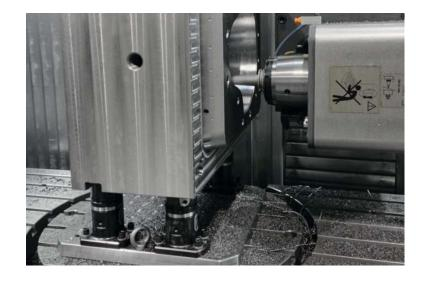
2 basic modules with a centring clamp adapted directly to a zero-point clamping system.
