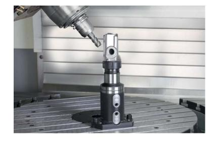
Gearbox housing mounted on 3 basic modules, 3 add-on modules and 3 reducer adaptors. The cast housing is secured to the reducer adaptors by means of socket-head screws.
