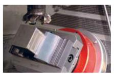
The Self Centering Vise 148 is made of rust-resistant material. All components are hardened. Highly stressed parts are specially surface-coated for increased durability.
