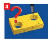
**04** | Diameters or sections can be quickly checked using simple measuring macros.
