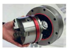
The three-jaw chuck is inserted. Both run-out and concentricity are repeated to an accuracy of 0.002 mm.
