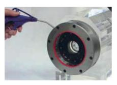
The chuck integrated with the machine spindle is opened with compressed air, either through an air-gun or through a fixed air supply.
