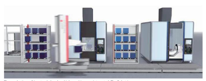
The production cell is extended and multiple machines are integrated. The Robot is equipped with a rail, additional magazines and a loading station. The initial investment is still used and extended, but now the production cell has the original capacity several times over.
