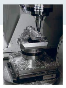
No matter how many chips, the Self Centering Vise remains clean at crucial points such as the spindle and guides.
