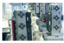
Variable use of tombstones. The MTS system provides an interface to fixtures and vises. Refitting takes no time at all.
