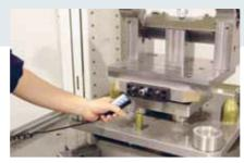
Each pallet is equipped with an EWIS™ identification chip. So you always have an overview of all magazine positions and pallets.
