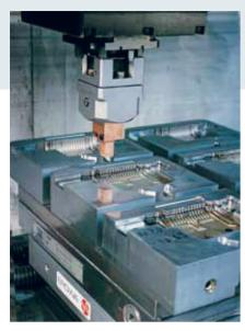
On a clamping surface of up to 500 x 500 mm, even large workpieces or fixtures can be attached to the UPC pallet without any problems.
