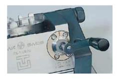
ITS S rapid-action chuck, able to rotate round 360°, indexing vernier 5 minutes (0.08°).
