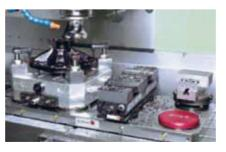
Various jobs can be done on one machine. Express jobs can easily be placed in between. Resetting the clamping equipment only takes a few seconds.
