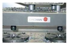
MTS chuck, able to automate. During the workpiece change, the contact surfaces are cleaned automatically.
