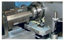
Horizontal chuck on a dividing head.
