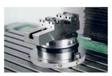
ClampSet vise on ITS pallet. Positioning to  $\mu$ -accuracy and ready for use within seconds.
