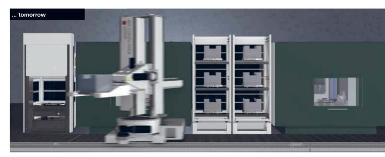
**Expand as needed** – More machines are added. The robot is equipped with rails and additional workpiece magazines. The initial investment is used further and supplemented. The capacity of the production line is multiplied, and more unmanned shifts can be realized.
