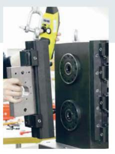
MTS chuck integrated in the mineral cast cube. In combination with the EROWA CleverClamp tooling system - a crucial production factor.
