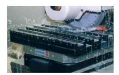
The UPC on the machine table constitutes the interface with the workpiece carrier. Resetting takes next to no time, and production can resume.
