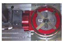
Gaskets protect the chucks and ensure secure automatic loading.
