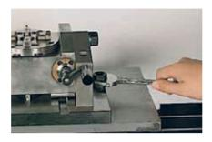
The EROWA Sine Dividing Head ITS is easy and quick to fit on the machine table, with only two bolts.
