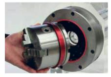
The base chuck is opened and the threejaw chuck is removed.
