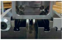
All moving parts of the self centering vise are protected.
