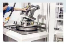
01 | A loading station is available to facilitate the setup and preparation of heavy parts.
