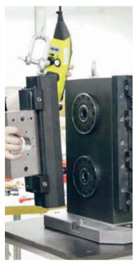
The CleverClamp base rails have holes on both sides to attach eye bolts.
