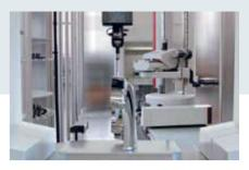
**03** | The handling facility serves the measuring station with manufactured products for interim and final checks.
