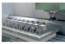
Short set-up times with flexible clamping elements: EROWA ClampSet vises on UPC grid pallet.
