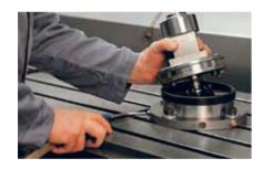
Clamped with  $\mu m$ -accuracy with one movement of the hand.
