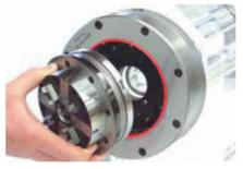
The palletized EROWA ITS chuck is inserted. The contour of the pallet completely seals off the spindle.
