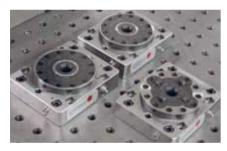
MTS single base plates are quickly installed and ready to use. Fit on machine tables with R50 and 63 mm hole grid and 100 mm T- slot spacing.
