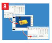
**08** | PreSoft XP is seamlessly integrated in JMS® Pro. The presetting function is activated by a mouseclick. The offset data that have been recorded are automatically transmitted from the measuring station into the JMS® Pro system.
