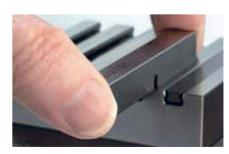
Simple means fast – changing jaws in no time and without any tools.
