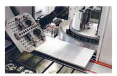
The chucks are completely sealed against ingress of coolant and chips. The contact surfaces are cleaned automatically and thoroughly with air.
