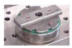
All axes, X, Y, Z and the center are checked with the same alignment plate.
