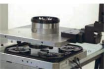
Universal combination of EROWA clamping systems with automatic handling.
