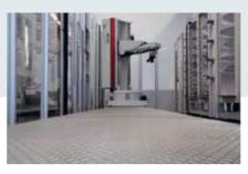
**02** | The stable linear rail is extended to the required length in segments.
