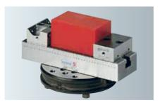
A fixture with Base 220 on an ITS pallet ø 148 mm.
