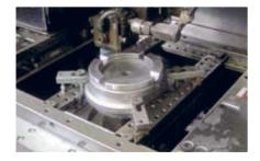
Special mounting for cylindrical parts. Mounted to the pendulum holder, the workpiece is adjustable in three axes.
