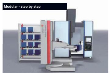
The first step is to equip the machine is such a way that most of the night hours can be utilized. One magazine is sufficient for this; with an average machine time of 30 minutes per workpiece, 5 hours can be put to productive use in this way.
