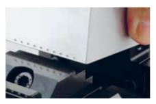
Clamping of workpieces with stamping technology at the minimum clamping height of 3mm.
