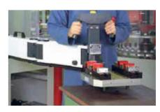
Lifting the pallet from the transport system.
