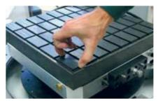
Thanks to the medium duct between chuck and pallet, workpieces may be clamped pneumatically, hydraulically or with a vacuum.
