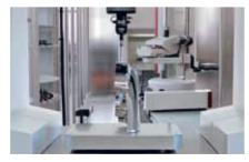
Using the automation kit (option), the CMM Qi can be loaded by an EROWA robot. The CNC control allows automatic quality measurements.
