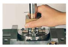
The workpiece is clamped with the precision of the ITS tooling system, with a repeatability of 0.002 mm.
