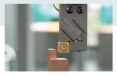
Simply ingenious: the 2D edge probe (EROWA patent) enables you to make the necessary measurements on radii, edges, corners and oblique surfaces.
