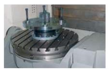
Another advantage: the workpiece or the fixture can be fitted directly on the PC pallet 210.
