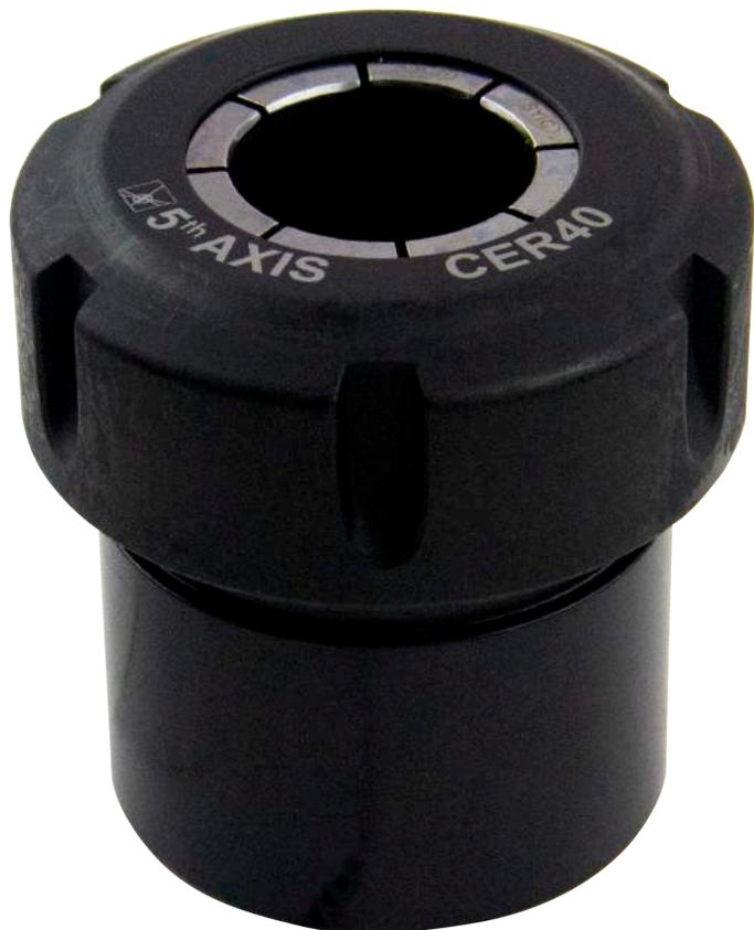
The CER40 is a quick and efficient fixture for holding round stock. The collet utilizes your existing set of standard ER40 collets allowing you to clamp different diameters of stock. The body is manufactured from hardened alloy steel.
