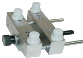
5 ALUMINUM CASE VISE Four plastic posts prevent damage. Posts can be set in different positions to hold various cases.
