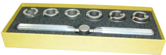
2 BERGEON KEY SETS For opening oyster cases manufactured by Rolex. Contains wrench and six milled chucks in the following sizes: 18.5, 20.2, 22.5, 26.5, 28.3 and 29.5 mm.
