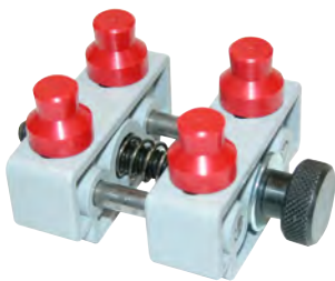
3 BERGEON JAXA CASE VISE Has plastic posts to prevent marring. Posts are removable and can be set into different positions for different cases. Opens and closes with large knurled knob. Plastic frame fits into bench vise.
