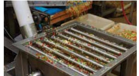
**Grate Magnets** used in food preparation at Better Baked Foods. Grate Magnets provide powerful, permanent protection against fine and tramp iron contamination.
