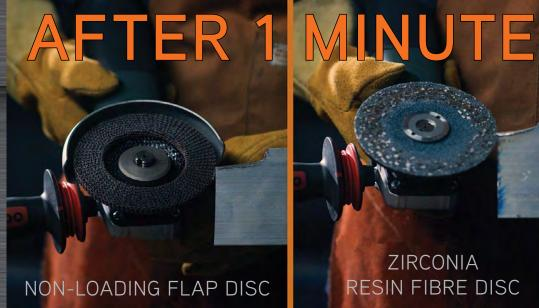
ZIRCONIA RESIN FIBRE DISC
