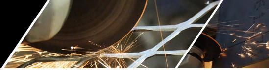
LIGHTNING is the "thinner" version of the High Energy formulation, it has the same great performance along with a slightly faster cutting speed and a smaller cut-line in the material being worked on. With a thinner profile, Lightning wheels are a bit more flexible for getting into tight recesses.
