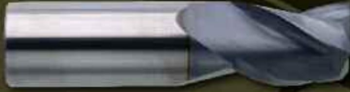
The ALDH is the 3 flute rougher of choice in most cases for optimizing metal removal rates. Our double helix geometry allows full engagement cuts at high feed rates. Feed rates of 50% higher than traditional two flute roughers provide a conservative starting point when calculating IPM.
