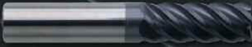
Our MH series is the tool of choice for finishing and light profile roughing in ferrous materials. The odd number of flutes disrupts unwanted harmonics. Our medium helix provides an optimum shear angle to aid chip evacuation. We have a full offering of square ends, corner radii, lengths and coatings to fit nearly any profiling operation.
