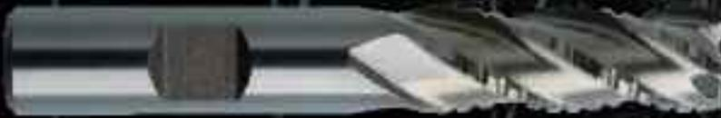
We have consolidated the Brubaker Starchip and Fastcut Ruff-N-Touch series into our Ti35. This is a multi-flute, 35 degree helix end mill aimed squarely at roughing or roughing/finishing in titanium and stainless steel alloys. This is a tried and true Aerospace workhorse made to NAS specifications. All tools are supplied as center cutting.
