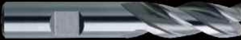
These three flute, M42 tools are manufactured with a 35 degree helix and radial relief on the OD. The result is an exceptionally strong cutting edge as well as superior finish on aluminum and non-ferrous materials. All tools are supplied as center cutting.
