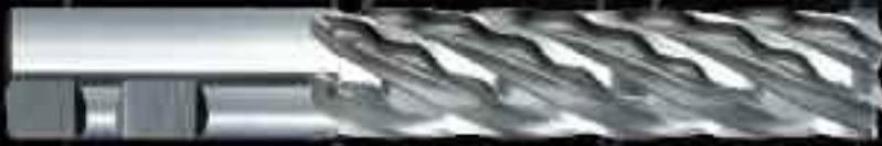
Our original Crest-Kut® end mills are a time proven design for superior metal removal rates combined with excellent finish in titanium and ferrous alloys. The sinusoidal wave form minimizes vibration and generates a chip form that improves evacuation and minimizes chip re-cutting. Excels in both peripheral and slotting operations. All tools are supplied as center cutting.
