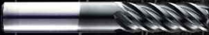
Our WM series end mills were designed specifically for finishing in titanium and exotic ferrous alloys. These end mills have a 45 degree helix for enhanced shearing action and a powdered metal substrate for superior wear resistance and tool life.
