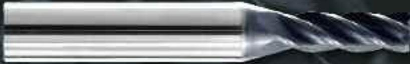
The extended reach design incorporates the proven geometries of the SSI-4 to allow for deep pocket roughing and finishing. The necked shank on these tools minimizes deflection during deep-reach milling operations.
