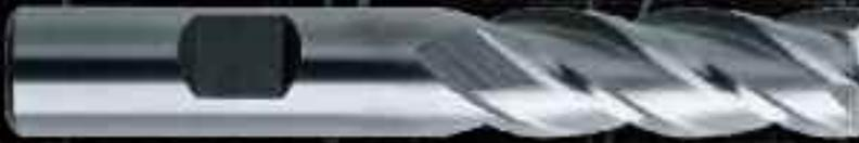
These end mills were formerly known as Brubaker SST Series. Our TiF35 series are intended to provide an outstanding finish in titanium and other exotic ferrous alloys. They are manufactured to NAS 986 type 46 and 66 specifications. All tools are supplied as center cutting.
