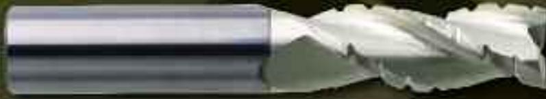
The ALDH-C is designed for very aggressive roughing in aluminum and non-ferrous materials. The chip breaker geometry allows for ease of chip evacuation and reduces cutting forces. These tools perform best when used with high performance milling chucks, or shrink-fit holders.
