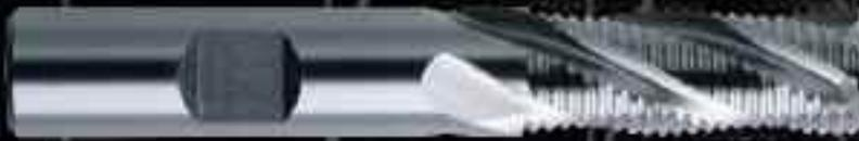
These end mills are intended for your most challenging roughing applications in titanium and ferrous alloys. The fine pitch serrations create smaller chips and aid in evacuation. Powdered Metal substrates provide an excellent balance of toughness and abrasion resistance required to machine medium to medium-hard materials. All tools are supplied as center cutting.
