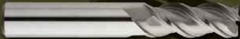
Our Tri-Power<sup>3</sup>® is a patented, three flute end mill for roughing and finishing in aluminum and non-ferrous materials. The high shear, 45 degree helix and patented flute form dramatically enhance chip evacuation under aggressive feed rates. The Tri-Power<sup>3</sup>® has beaten the competition in metal removal rates and cycle time reduction in test after test.
