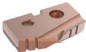
150° Structural Steel For material over 7/16" thick and for reduced exit burr
