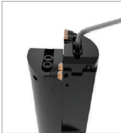
Step 5: Tighten the mounting screws on the cartridge to 11-14 ft-lbf (15-19 N-m).
