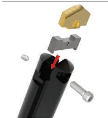
Step 1: Position the adapter into the holder.
